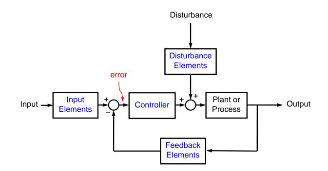
Each box will then contain the transfer function of the element contained in the box.
