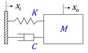
**Exercise**: Noting that the input to the above system is a displacement, show that the **transfer function** for the system is given by
