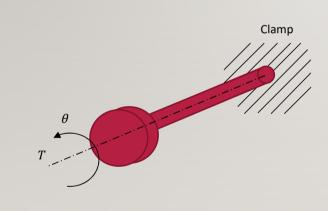
Derive expressions for the transfer functions that relate input torque T(t) and output angular displacement θ(t) of the torsional system shown for the following cases:
